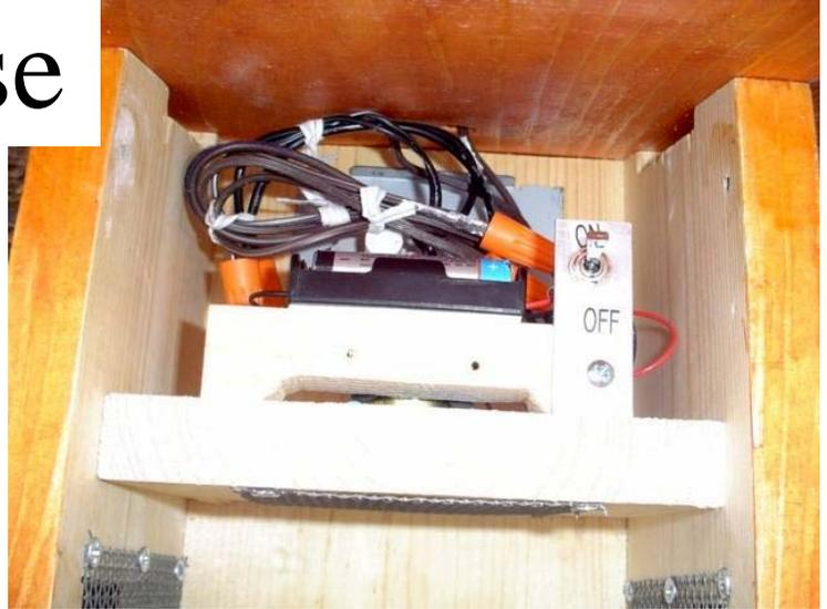
A solar panel embedded in the roof of the nest box powers a miniature solar fan motor and also charges a single 1.2 V 2000 mAh AA Nickel Metallic Hydroxide (NIMH) battery that serves as a backup source of power. A single pole, single throw (SPST) switch secures the fan motor when it is not needed or maintenance is required.
